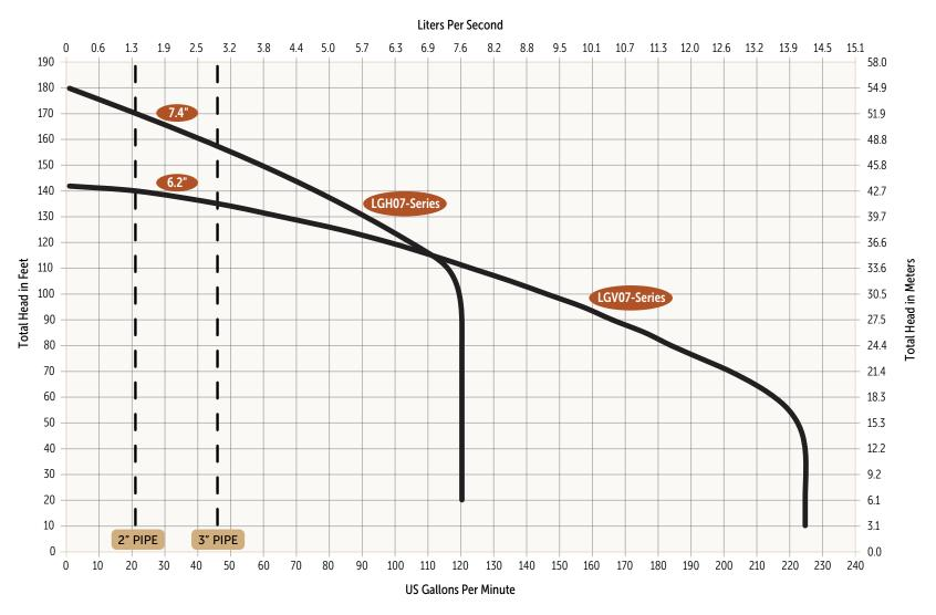
Pumps must operate within the proper range shown on the performance chart. It is the responsibility of the end user to ensure this requirement is met. Pumps operating outside the recommended range are prone to damage, excessive vibration, cavitation, poor efficiency, and may exceed nameplate amperage.
